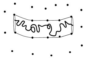
FIG. 6. Chain trapped in fixed network of obstacles created by other chains. Circles, topological constraints imposed on motion of chain by other molecules. Thin lines, effective tube in which chain is free to move.
